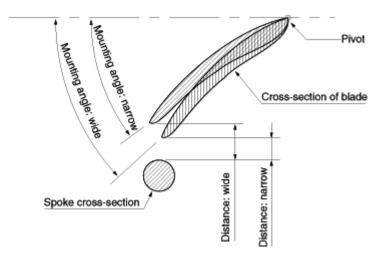
Fig. 6 Positional relation between cross-section of blade and spoke
