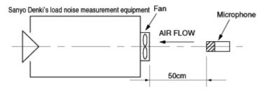
Fig. 5 Method of load noise measurement
