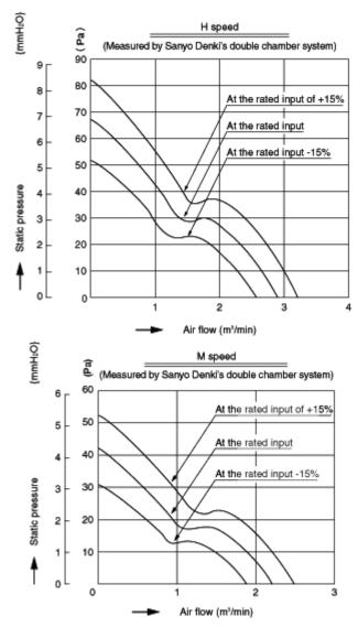
Fig. 3 Example of air flow versus static pressure characteristics of the low noise "SAN ACE 120L"
