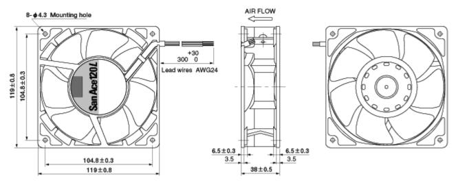
Fig. 2 Dimensions and specifications of the low noise "SAN ACE 120L"
