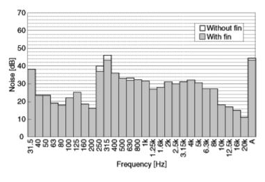
Fig. 8 Noise analysis data of 1/3 octave band Static pressure = 20 (Pa)
