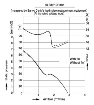
Fig. 7 Air flow versus static pressure and noise characteristics
